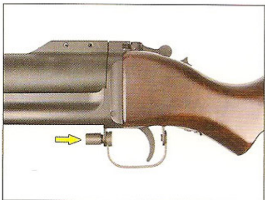
3. The trigger guard can go sideways after release the detent button.
