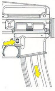
Press magazine catch button and remove the magazine from lower receiver.
