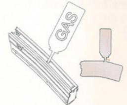
Hold the magazine sideway and let the gas valve hole facing up. Charge the magazine with 134A gas or green gas. Make sure the gas bottle and the magazine are perpendicular when charging.
