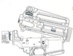
Install the upper receiver back on with the lower receiver, ensure the selector lever is pointed to safe.
