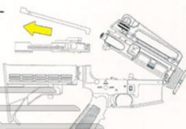
Pull back charging handle and bolt carrier. Then push front pivot pin out, separate upper and lower receivers.
