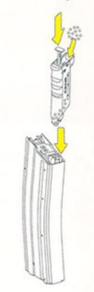
Align the BB loader outlet with the magazine opening. Press loading rod to load BB into the magazine.
