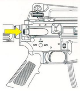
Press the forward assist button to make the piston go forward if needed.
