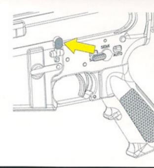
When finish shooting the loads, the bolt will be staying at the bolt stop (it will not stop if the magazine is adjusted to the empty shooting mode.). Press the upper part of the bolt catch indicated by the arrow, the bolt will be able to go back to closing position.
