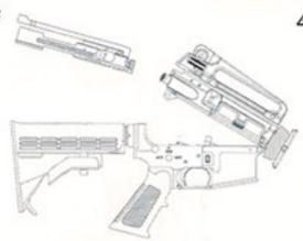
Insert the charging handle and bolt carrier together into upper receiver.
