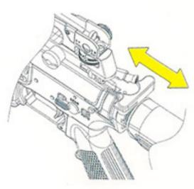
Preparing to fire, pull and release the charging handle to load.
