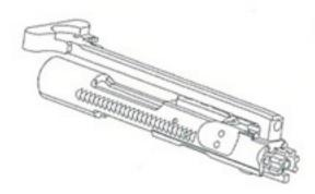
Place charging handle on top of the bolt carrier as shown.
