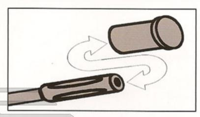
Always attach the protective plug to the gun muzzle.
