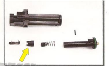
Finally, take the valve and other parts out. Replace the valve blocker and reassemble the rifle (Refer to page 5).
