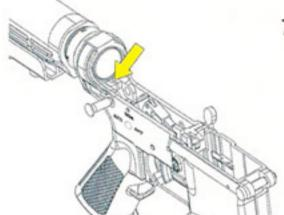
7. Depress buffer retainer and release buffer from stock tube.
