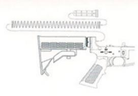
First to install the recoil spring and buffer back by depressing the buffer detent and slide the recoil spring and buffer back into stock tube. Release buffer detent afterwards.
