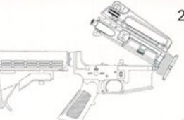
Engage receiver pivot pin to join upper and lower receivers.
