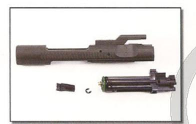
Take the loading nozzle out from bolt carrier.
