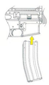
Insert the loaded magazine into the rifle.
