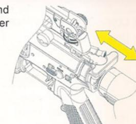
Pull the charging handle backward, check receiver and chamber to ensure there is no ammunition in the rifle.
