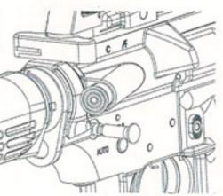
Slide the takedown pin back on and make sure it goes through the upper and lower receiver.
