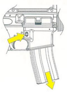
Press the magazine catch button to release the magazine.
