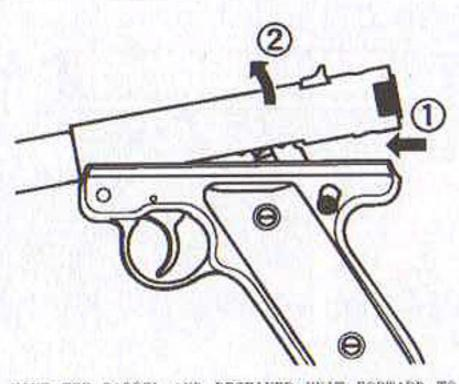
MOVE THE BARREL AND RECEIVER UNIT FORWARD TO FREE IT FROM THE INTERNAL BOOK AT THE FRONT OF THE FRAME.
