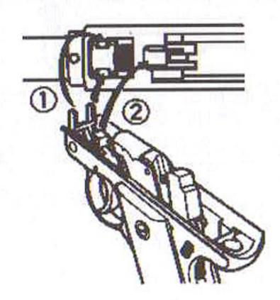
PLACE THE BARREL/RECEIVER ASSEMBLY ON THE FRAME.
