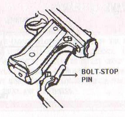
PLACE THE MAINSPRING BOLT-STOP PIN INTO THE BASE OF THE RECEIVER AND THROUGH ITS HOLE IN THE BARREL.
