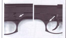
PRESS THE DISASSEMBLY LATCH RELEASE AND ROTATE THE DISASSEMBLY LATCH CLOCKWISE UNTIL IT STOPS.
