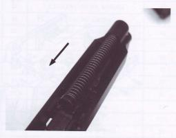
REMOVE THE RECOIL SPRING GUIDE AND SPRING.
