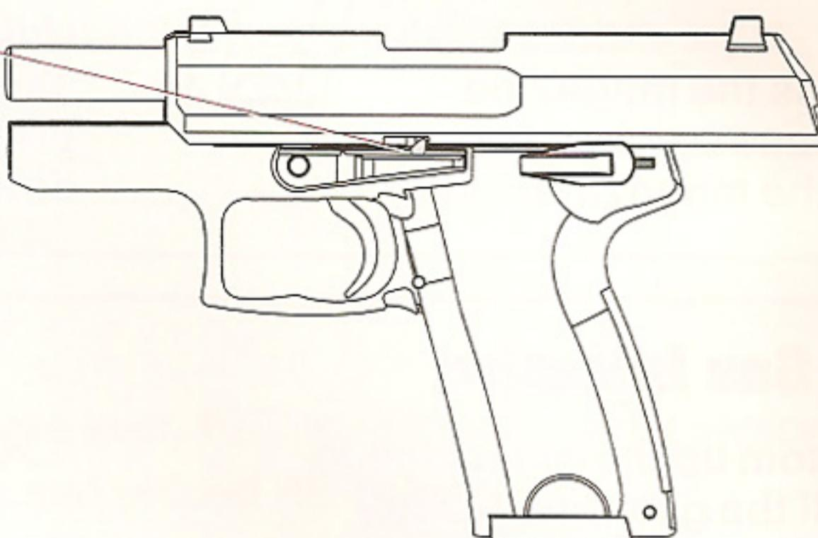
While first load for firing, pull the slide backward to a specific position to load the bullets in the firing chamber, then ready to fire.
