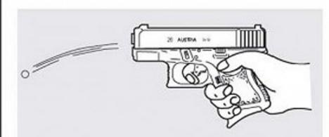
After a long and continued firing practice, the low temperature of the magazine will cause a reduced gas pressure as well as the low velocity of pellet. It is a normal condition and not a trouble.
